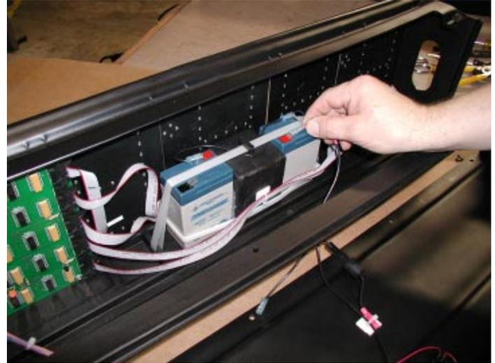
Install the two power wires
