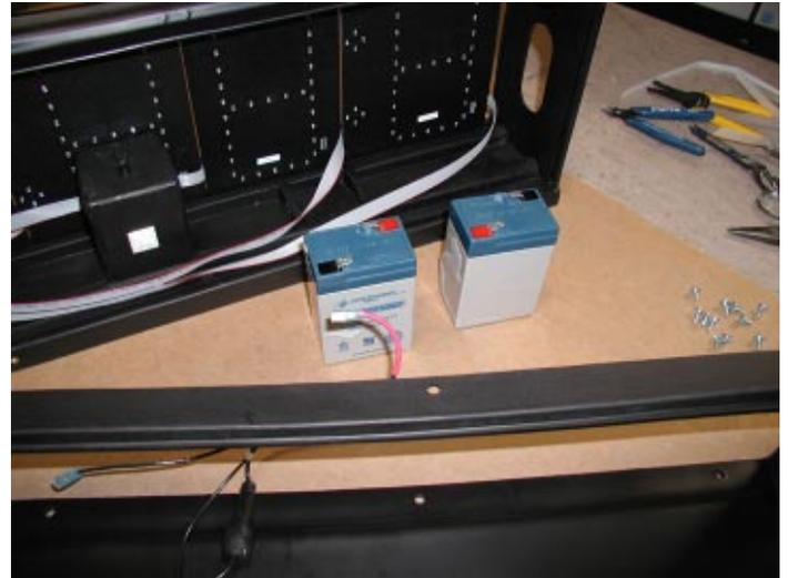
Remove the two batteries
