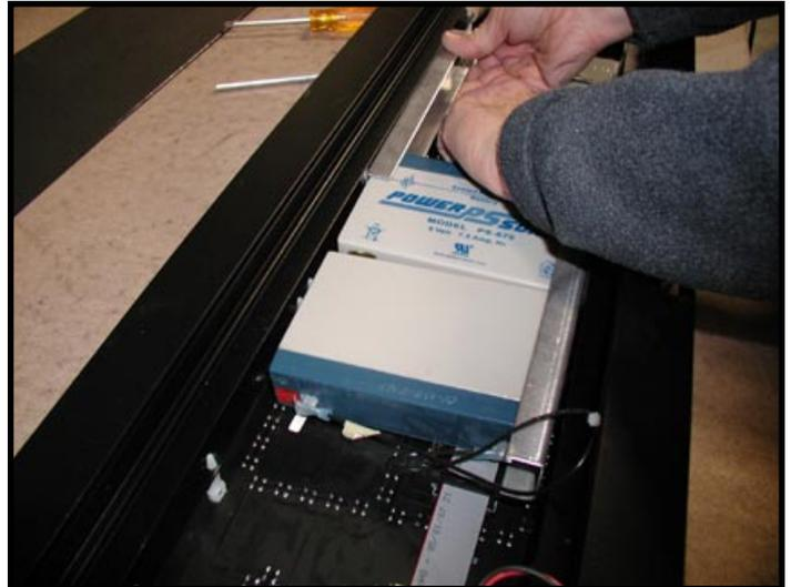
Remove the battery clamp top channel.
