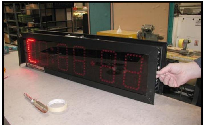
Test clock operation before final assembly.
