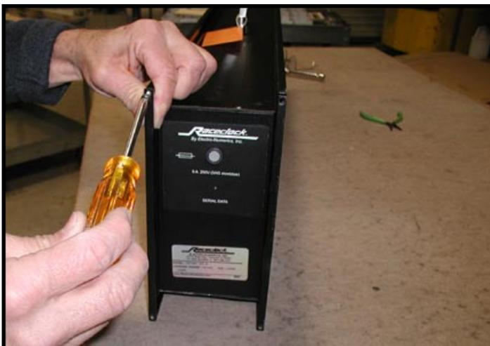
Replace the two top (smaller) corner screws.
