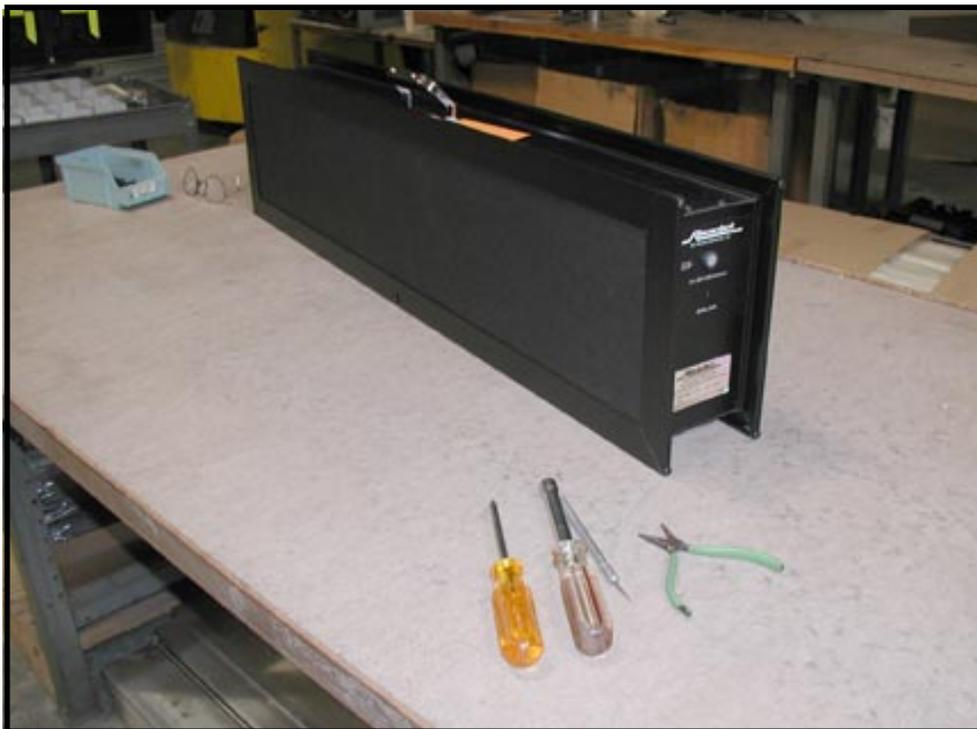
2) Using a philips screwdriver, remove the 8 screws on the end of the clock that has the panel mount fuse. With the clock upright, remove the four screws on the top (2A), turn the clock over (2B) and remove the 4 screws on the bottom (2C & 2D).
