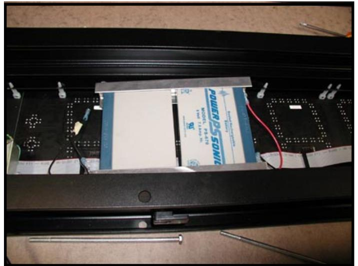
Carefully note the orientation of the batteries.
