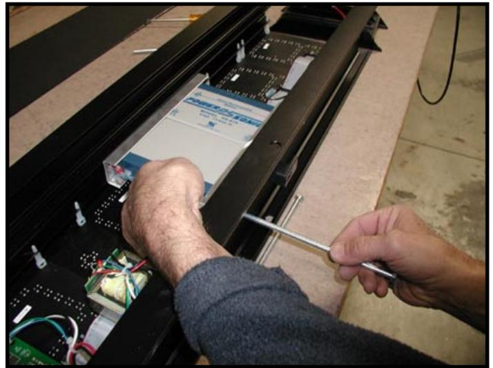
Remove the first battery clamp bolt.
