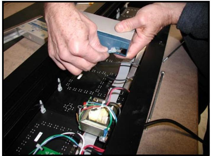
Remove the battery power wires.
