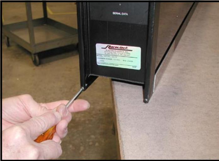
Replace the two bottom (smaller) corner screws.
