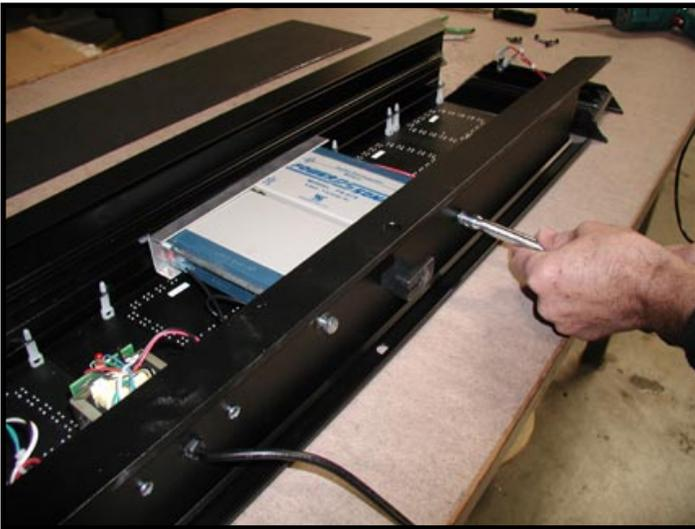
Remove the second battery clamp bolt.
